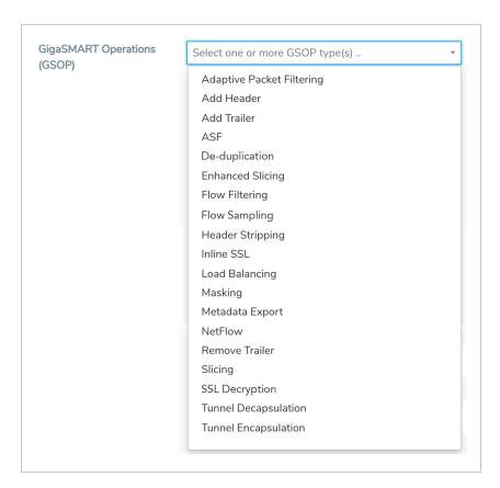
In GigaVUE HC Series hardware appliances, GigaSMART applications run on specialized GigaSMART advanced-processing engines and perform functions on the traffic in real time to improve network visibility and improve security and other tools' performance. Access the GigaSMART advanced processing engines from any GigaVUE® HC series node, without port- or card-based restrictions, and combine GigaSMART engines to manage higher traffic loads and optimize for specific applications.
